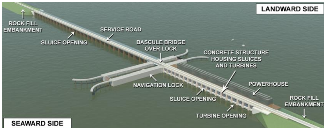
Figure 21: Tidal Power Project, with navigation lock, © WSP
