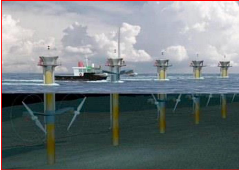
Figure 9: An illustration of a tidal fence (reproduced from IT Power)
